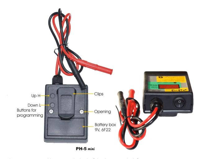
There are two round buttons at the back of the device, on the left.
